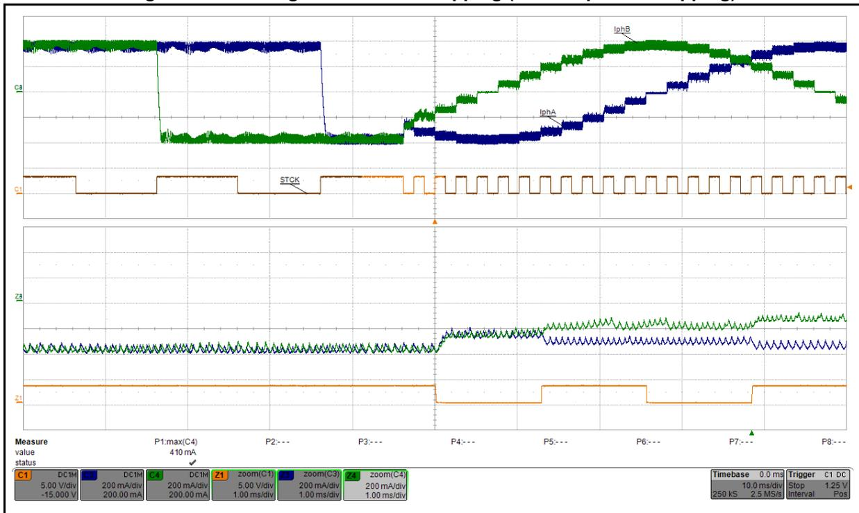
Figure 7. Switching to full-step (1/64<sup>th</sup> step microstepping)
