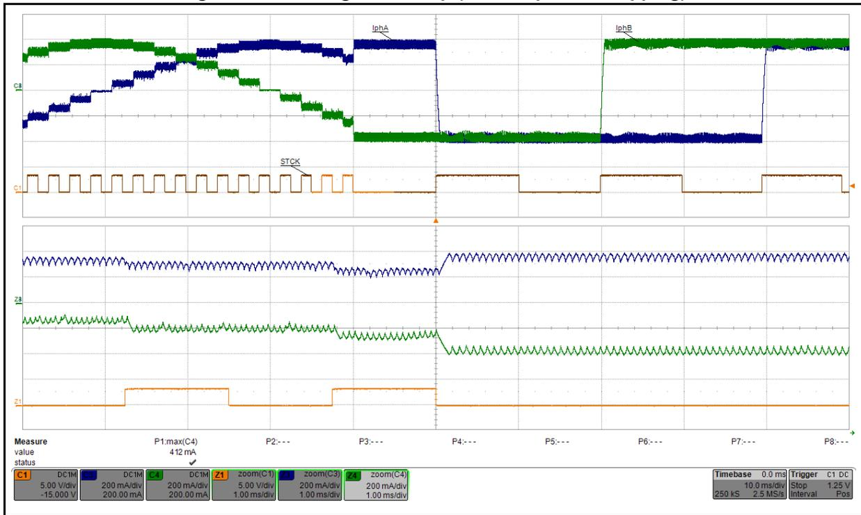
Figure 6. Switching back to microstepping (1/8<sup>th</sup> step microstepping)
