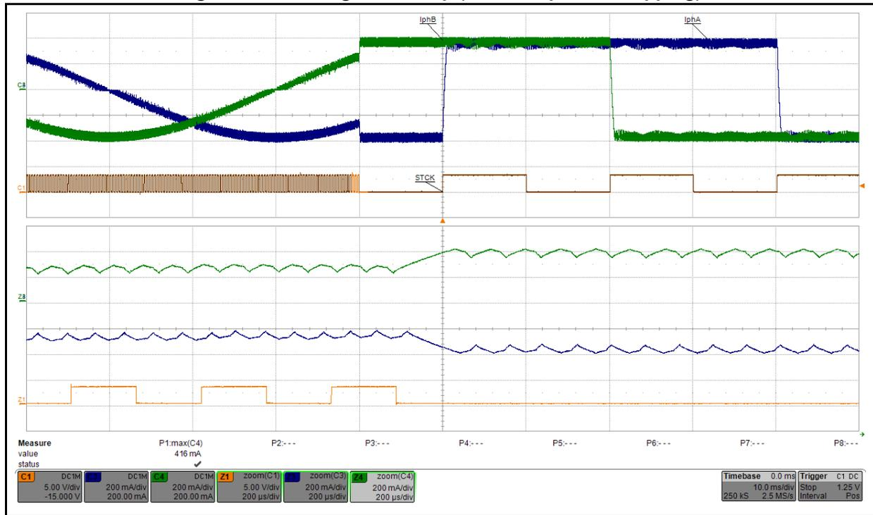
Figure 8. Switching back to microstepping (1/64<sup>th</sup> step microstepping)
