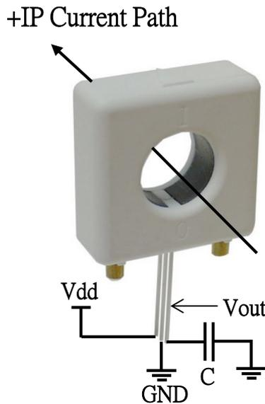
Capacitor **C**(0.01uF~0.1uF) is recommend to be connected between Vout and GND to reduce output noise.
