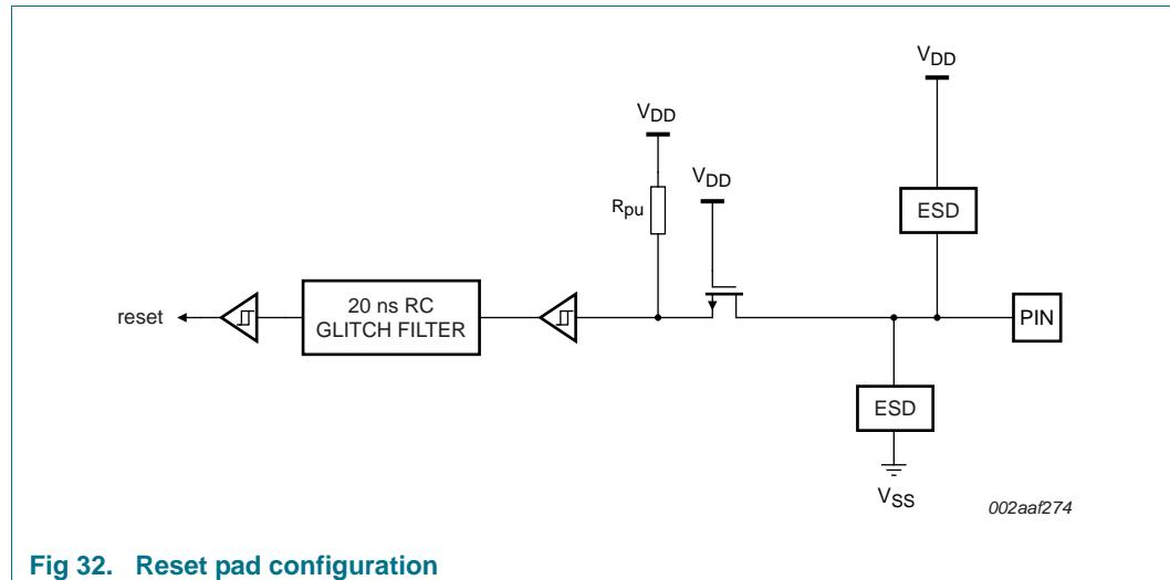
**Fig 32.** Reset pad configuration
