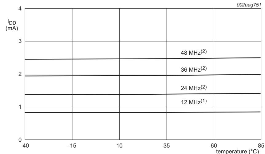
**Fig 11. Typical supply current versus temperature in Sleep mode**
