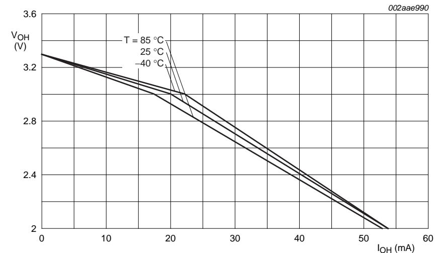
Conditions:  $V_{DD} = 3.3$  V; on pin PIO0\_7.
