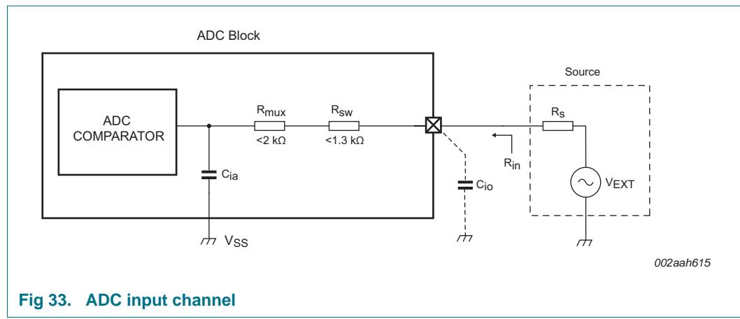
**Fig 33.** ADC input channel
