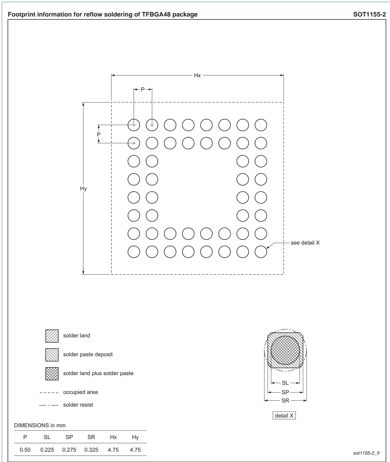
Fig 42. Reflow soldering for the TFBGA48 package
