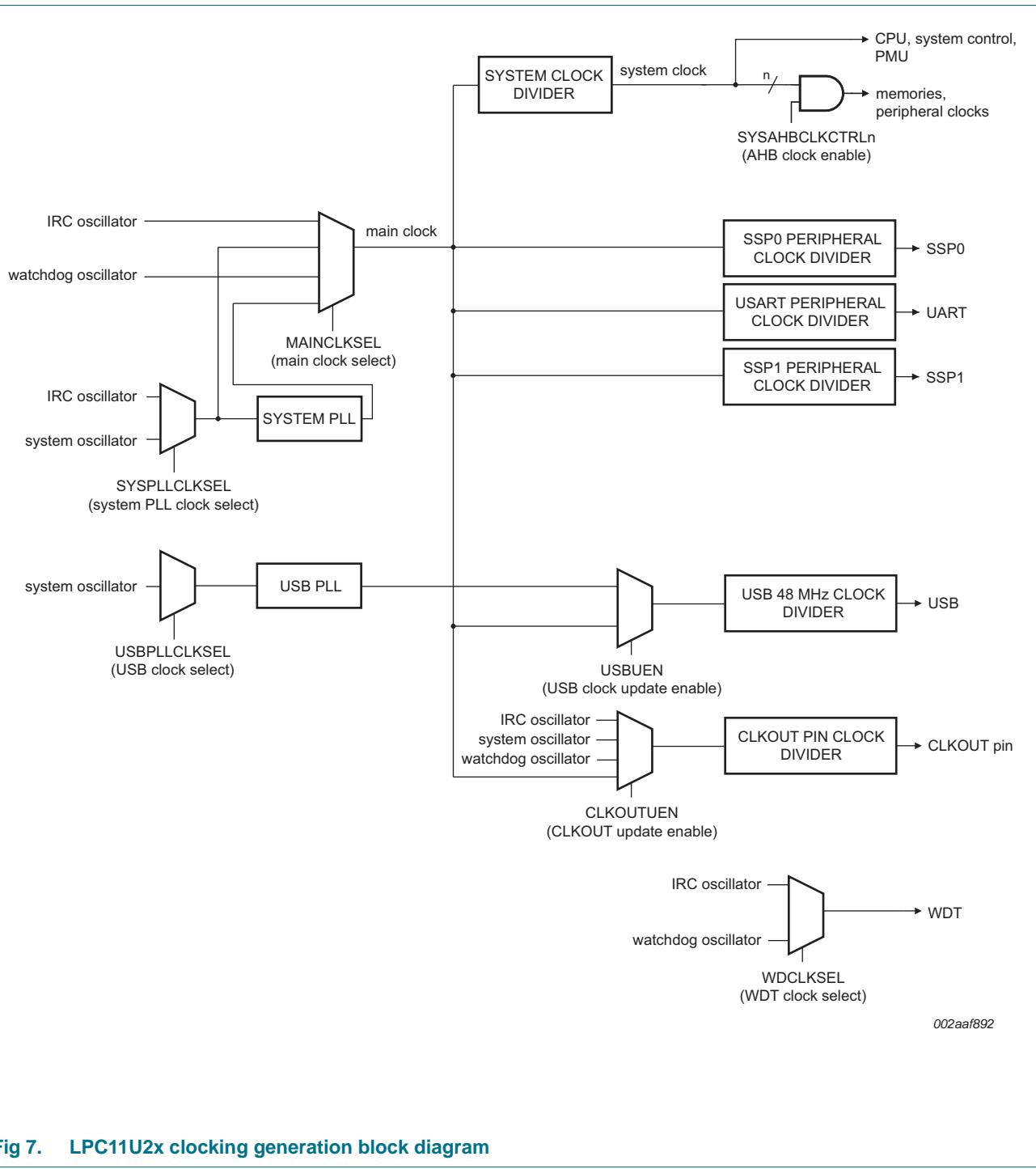
Fig 7. LPC11U2x clocking generation block diagram
