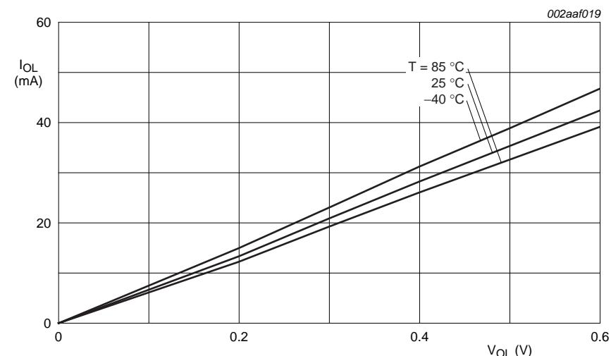
Conditions:  $V_{DD} = 3.3$  V; on pins PIO0\_4 and PIO0\_5.
