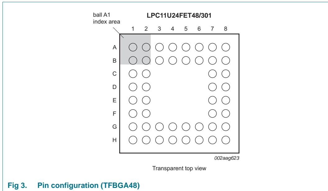
Fig 3. Pin configuration (TFBGA48)
