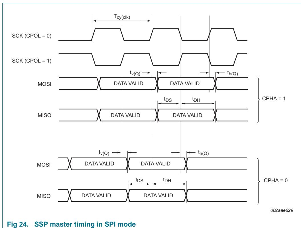
Fig 24. SSP master timing in SPI mode
