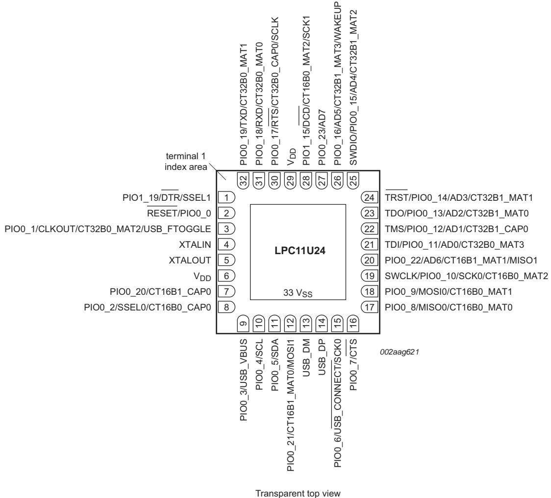
**Fig 2. Pin configuration (HVQFN33)**
