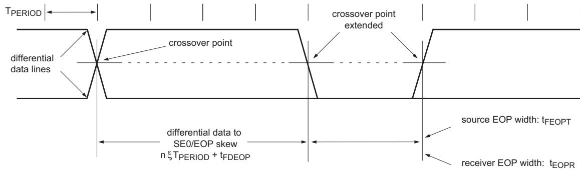
**Fig 26. Differential data-to-EOP transition skew and EOP width**
