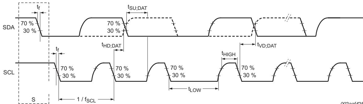
**Fig 23. I<sup>2</sup>C-bus pins clock timing**
