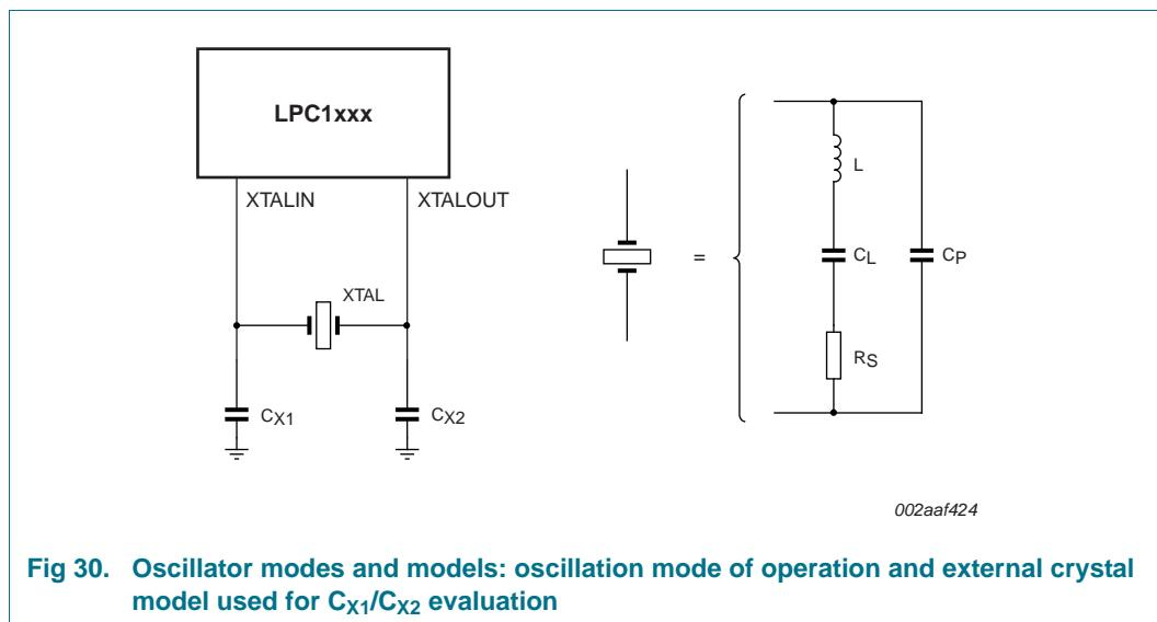
**Fig 30. Oscillator modes and models: oscillation mode of operation and external crystal model used for  $C_{X1}/C_{X2}$  evaluation**
