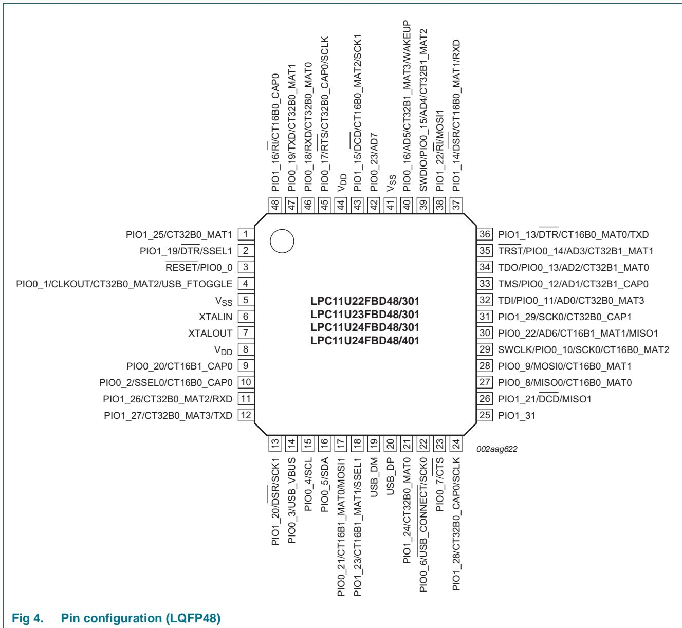
Fig 4. Pin configuration (LQFP48)
