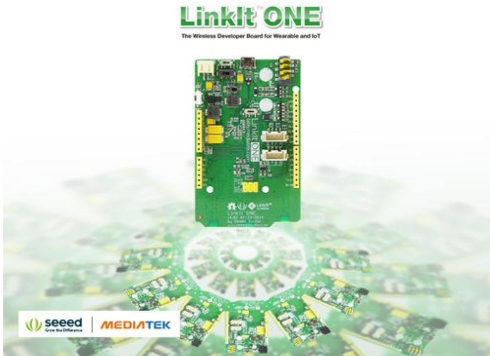
The LinkIt ONE development platform is an open source, high performance board for prototyping Wearables and IoT devices. It is based on the world's leading SoC for Wearables, MediaTek Aster (MT2502) combined with high performance Wi-Fi (MT5931) and GPS (MT3332) chipsets to provide you with access to all the features of MediaTek LinkIt. It also provides similar pin-out features to Arduino boards, making it easy to connect various sensors, peripherals, and Arduino shields.
