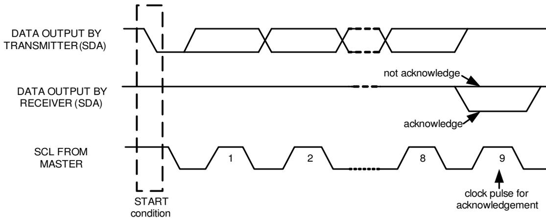
**Figure 10: Acknowledge on the I<sup>2</sup>C Bus**
