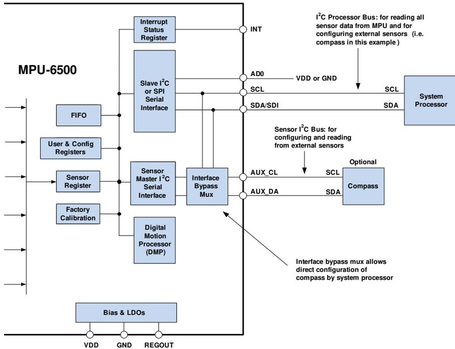
**Figure 6: MPU-6500 Solution Using I<sup>2</sup>C Interface**
