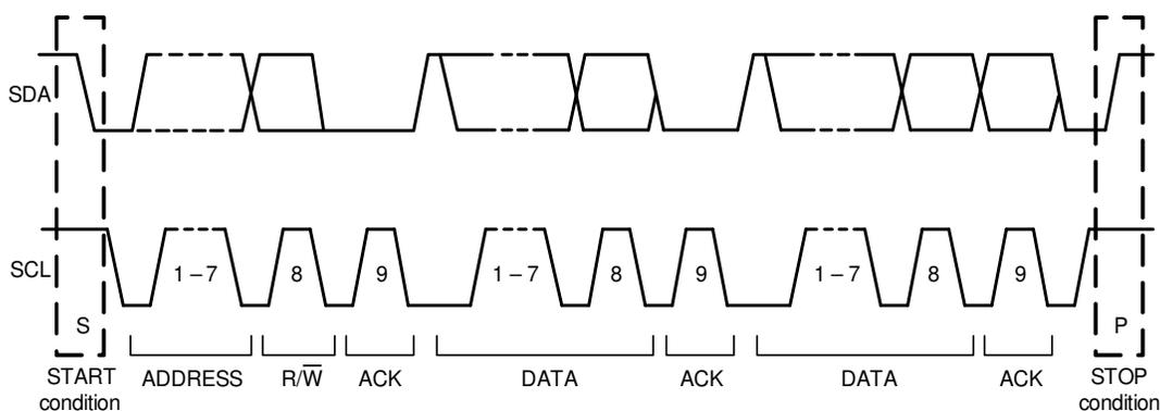
**Figure 11: Complete I<sup>2</sup>C Data Transfer**
