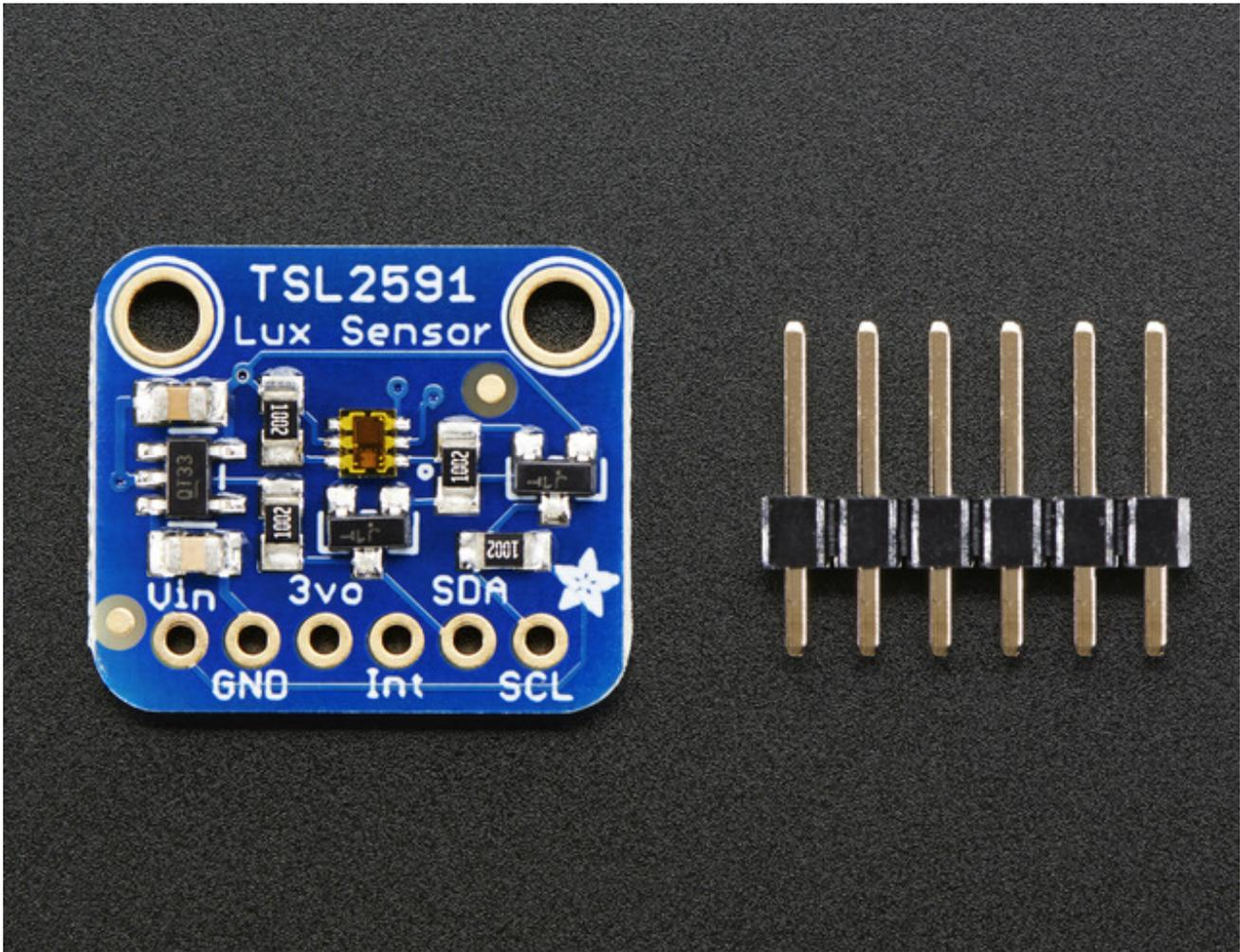
The built in ADC means you can use this with any microcontroller, even if it doesn't have analog inputs. The current draw is extremely low, so its great for low power data-logging systems. about 0.4mA when actively sensing, and less than 5 uA when in power-down mode.
