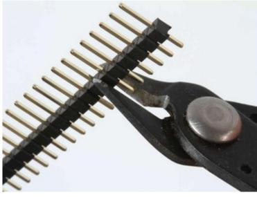
Cut the header strip to length if necessary and place it in the breadboard (long pins down!). Position the breakout board over the header.
