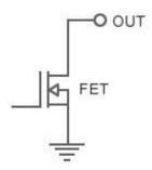
Since there is no internal connection to VCC, the open drain output does not put out a voltage like an Arduino GPIO pin. You have to provide your own external pullup. While this may seem inconvenient, the open drain configuration allows for a lot of flexibility. Since the output voltage is not dependent on the operating voltage of the breakout, you can use a variety of power sources. The FETs in the DS2413 are capable of switching voltages up to 28v and up to 20mA.
