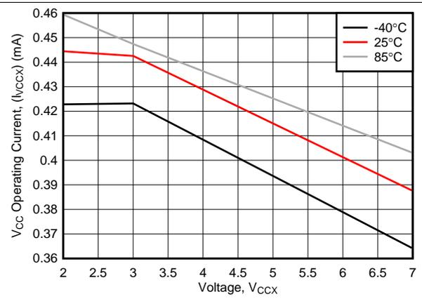
Figure 5. V<sub>CC</sub> Operating Current
